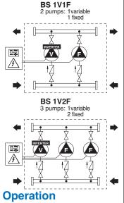
The control panel, with electronic card, manages the pump operation, the changeover of fixed speed pumps starting sequence Pumps starting is in a cascade sequence, with a signal from the pressure transducer. Constant pressure is guaranteed by the variable speed pumps, while fixed speed pumps start when the request is higher than the capacity of the variable speed pump. BS 1V1F
